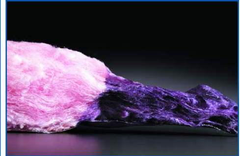
Fiberglass, when wet and compressed, loses a significant portion of its insulative value and over time could serve as a catalyst for mold, mildew and other unwanted bacteria.
