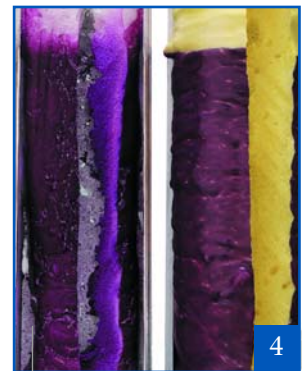
4 Samples were cut along a vertical cross section to assess the amount of absorption, wicking, moisture retention and foam shrinkage.
