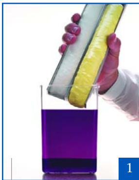
1 The fully cured foam samples were inserted halfway into a beaker filled with purple dyed water.
